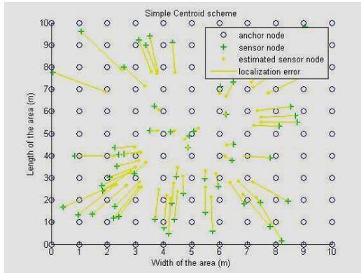
Fig 5. Simple Centroid Scheme Location error
