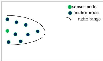
Fig 4. Sensor node near left border. The anchor nodes can be present on its right, top and bottom but not on its left.
